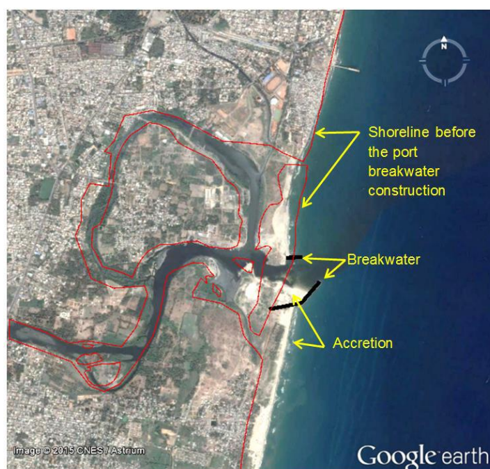
Fig.2. Status of shoreline before and after construction of Puducherry harbour (Source: NIOT)
