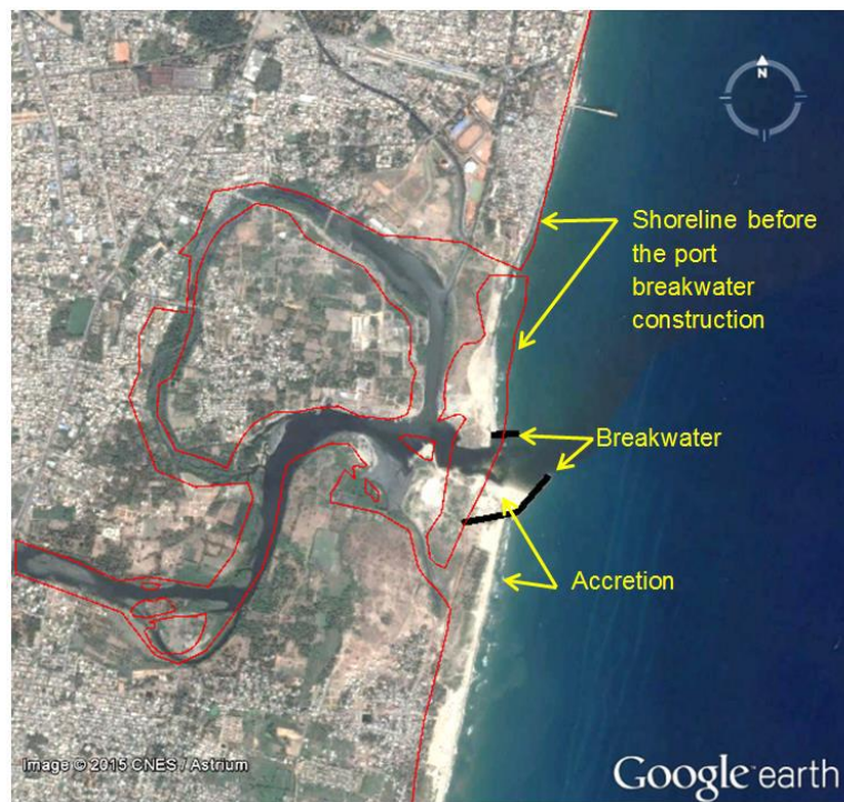
Fig. 4.2. Status of shoreline before and after construction of Puducherry harbour (Source: NIOT)
